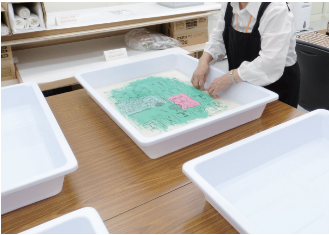
図4 短時間浸漬法：水を張ったバットに順に浸漬する Fig. 4 Short Duration Soaking Method: The artifacts are soaked one by one in a series of water-filled trays
